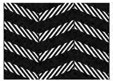
Figure 4: Globally isotropic structures with negative Poisson’s ratio (of Milton).
